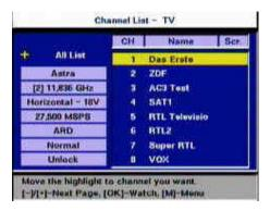
Press the **b**utton to show the channel list. A + for the main channel list or the "apple" symbol is indicated at the top left. The list can be changed by pressing the button again. Information relating to the received satellites, the polarization, the symbol rate, scrambling, favorite or standard channel and the parental control is provided in the column below the symbol. The column on the left contains information relating to the channel, the
